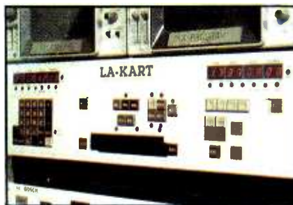
Shown is one of the interface panels. One panel is required for each pair of tape machines.
